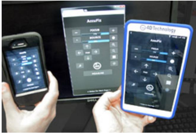
Figure 10. Remote controls for adjusting source diameter, focus, zoom and pan, and for taking a measurement, are available on-screen, on a dedicated remote, and through mobile devices.
